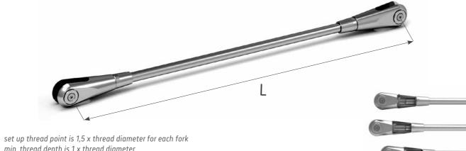
min. thread depth is 1 x thread diameter fork adjustment is 0,5 x thread diameter for each fork
